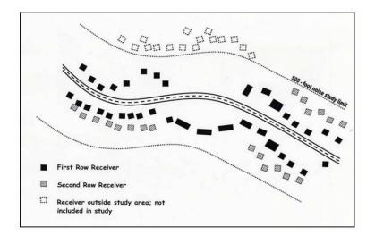
Step B: Identify the first row of receivers from the front and appropriate sides of the buildings. Note that the first row may be positioned at locations higher than the ground floor.
