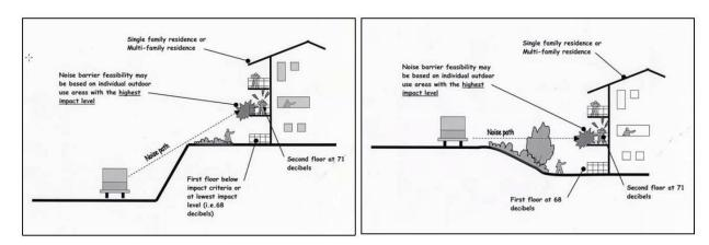
Step C: Identify the appropriate line-of-site for impacted receivers (please only count one receiver per story within the vertical column of the building).
